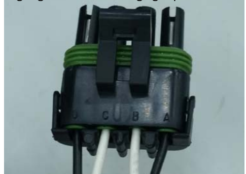
A– positive in B– ground in C– warning light ground D– warning light positive
