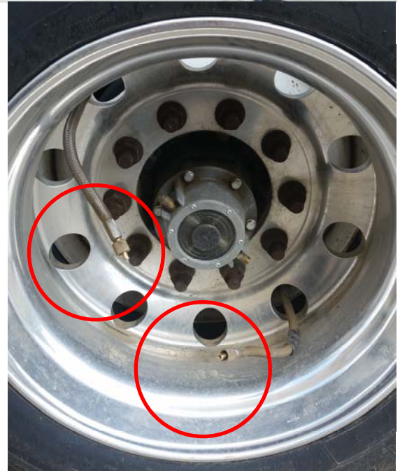
Soap check hose ends for backflow
