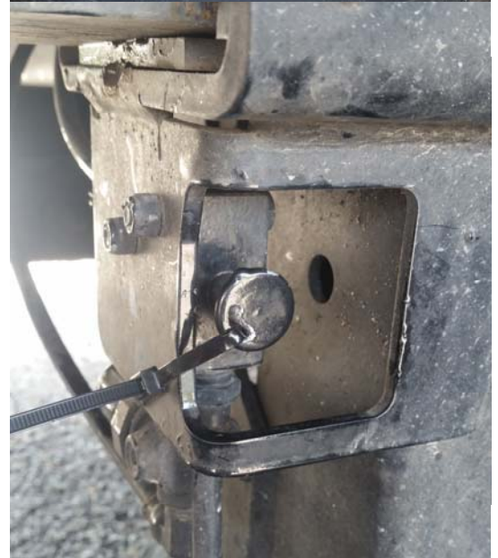
Push/pull valve vibrated out dropping trailer air tank pressure. This withdrew air from the Pressure Guard system turning on warning light. Pressure Guard system did not have a problem. Pressure Guard wheel hoses have check valves preventing tire pressure back-flow
